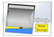
5 Degree Leanback Saves Water and Improves Bearing Life Bearing loads are much lower as the center of gravity of the load is moved closer to the bearings at the back of the cylinder during high speed extraction, reducing noise and vibration and extending bearing life.
