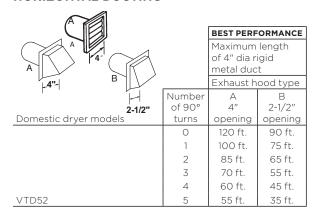
For every extra 90° elbow, reduce the allowable vent system length by 10 ft.
